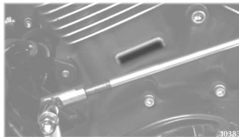
Engine identification number stamped on right side of engine
