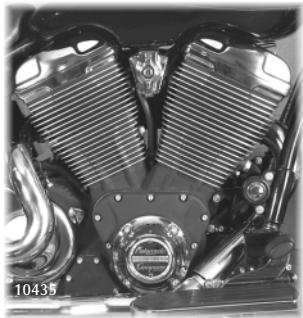
The heart of the Super X is its unique X-Twin™ engine. The 85 cubic inch displacement power plant features two dual overhead cam, four valve, opposed cylinders configured at a 50° angle. Each of the massive black cylinders blows into an exhaust system that mirrors the highway as it stretches rearward.
